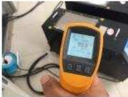
measure the temperature of Vietpro loadbank by infrared thermometer
